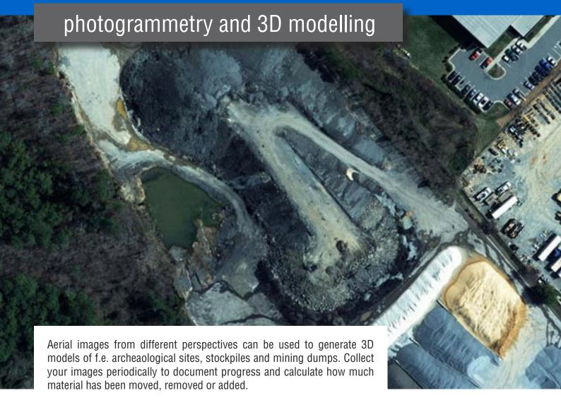
Close range aerial photogrammetry offers much potential for measuring features that can't or aren't being measured otherwise.
