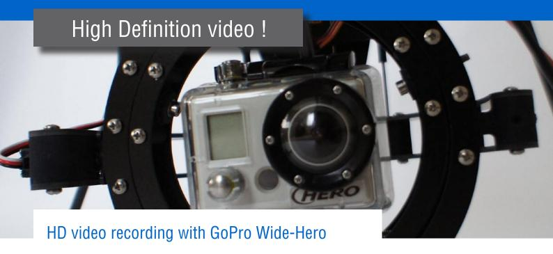
Ellipz designed a special gimbal for the GoPro camera. The GoPro HD Wide-Hero enables you to record in HD 1080p quality, everything is recorded in the highest detail. You also don't have to worry about recording times. It enables you to record up to 2,5 hours on 1 battery and up to 9 hours on a 32Gb SD-card.
